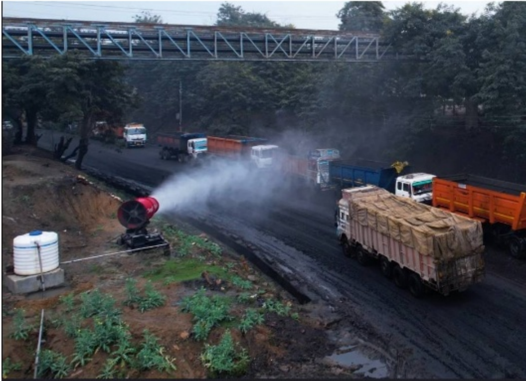
Fixed Fog Canon at Mine Barrier
